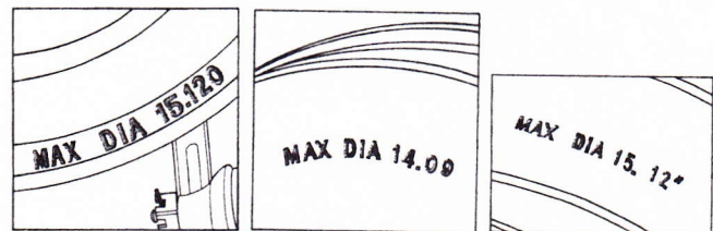
Figure 45-24 The drum's discard diameter is stamped on the drum.
