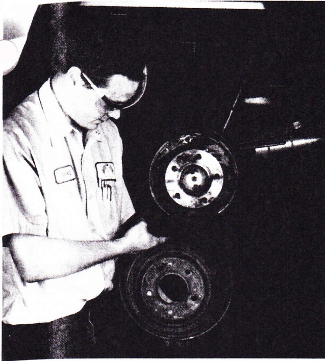
Figure 45-16 Carefully check the inside surface of the brake drum.
