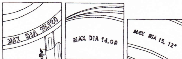
FIGURE 39-29 The drum's discard diameter is stamped on the drum.
