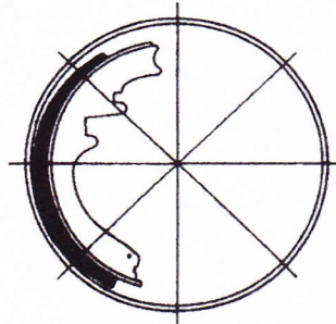
TYPICAL OEM OFFSET GRIND (FURNISHED ON NEW VEHICLES)
