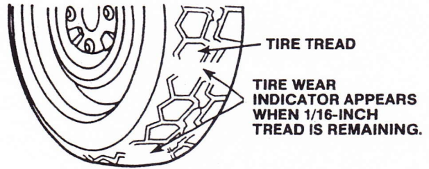
FIGURE 35-14 Tread wear indicators.
