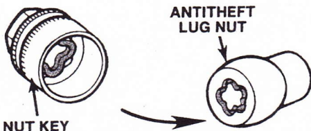
FIGURE 35-17 Circular keyway fits female slot of antitheft wheel lug nut. Courtesy of Ford Motor Company
